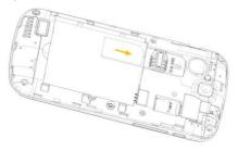
Insert the memory card into the metal slot with the metal contacts facing down until it clicks to the right position.
